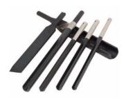
6. **Handles,** (For Thompson or Ellsworth **Small** Hollowing Tools) "17 Inch Ash Wood Handle" from www.woodturnerscatalog.com. Same as handle on Ellsworth Signature Gouge. Or "Hosaluk 18 inch Aluminum Handle". Steel handles, especially the Oneway handles are to heavy!
