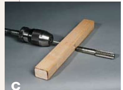
C Insert a \frac{1}{4} x 1\frac{3}{4} " bolt through the \frac{7}{16} "-square hole in the tap handle.
