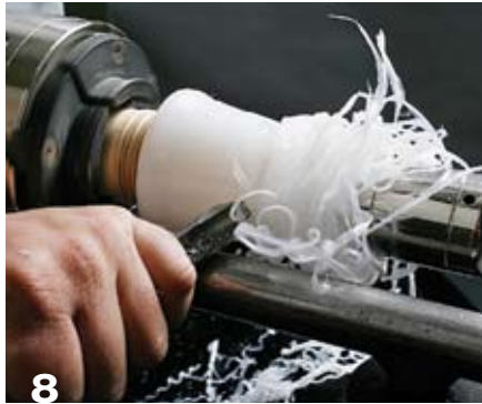
8 Ride the bevel while turning the cone shape with a bowl gouge.
