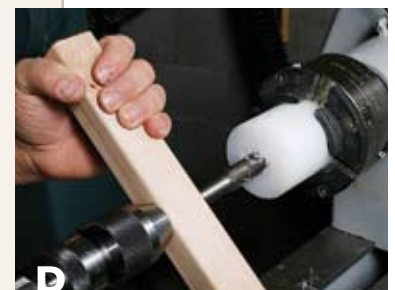
D Rotate the tap handle by hand while slowly advancing the tailstock.
