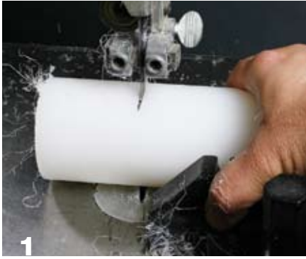
1 To avoid a catch at the bandsaw, support the UHMW cylinders with a miter gauge.
