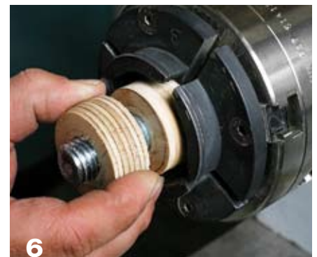
6 Use two ¾" plywood spacers to clear the jaws of the chuck.
