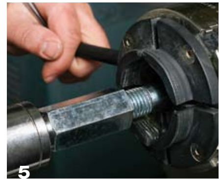
5 Mount a partially threaded 5"-long bolt (head removed) in a 4-jaw scroll chuck.
