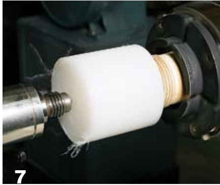
7 To keep things running true, keep the tailstock in place as long as possible.
