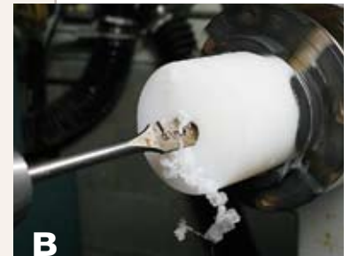
B Run the lathe slowly while advancing the \frac{5}{8} " spade bit into the UHMW stock.
