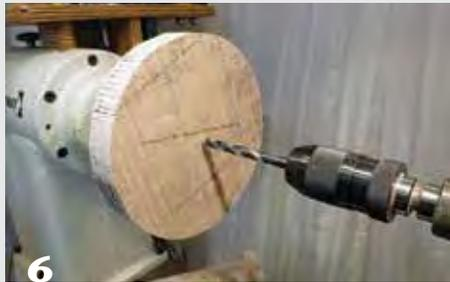
Drill a pilot hole for a screw chuck in the top of the base. Then turn a flat in the center 3" to 4" wide.
