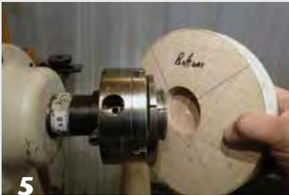
Mount the lamp base on your chuck by expanding the jaws into the hole on the bottom.
