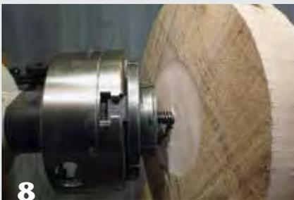
Mount the top of the base onto the screw chuck. The chuck jaws will register against the turned flat area.
