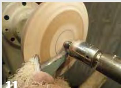
**11** With the base now re-mounted on the chuck in expansion mode, mark a  $2\frac{1}{2}$ "-diameter circle in the middle of the top. Create a concave area within this circle, then shape the remainder of the top.
