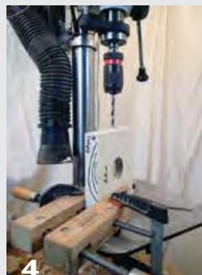
(3) Drill a ¾"-deep hole with a 2½"-diameter Forstner bit in the bottom center of the lamp base.
