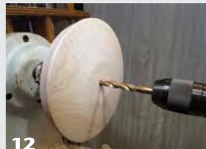
**12** Enlarge the center hole with a  $\frac{13}{32}$ " or  $\frac{7}{16}$ " twist drill to fully accept the  $\frac{3}{8}$ " OD lamp rod.
