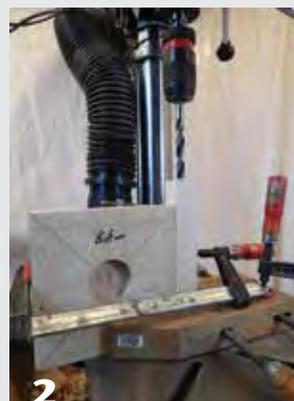
(1) A wooden hand screw clamp to your drill press table aids in accurate drilling. Use a square to double-check alignment before drilling all the way through the lamp shaft blanks.
