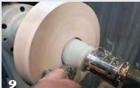
Use a bowl gouge and shear-scaper to turn the bottom of the lamp base. After truing up the outside edge, form a concave surface in the middle. A straightedge touching the outer edges indicates concavity.
