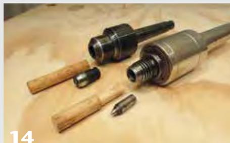
**14** Two alternatives for mounting dowels in the tailstock live center with center point removed. *Top*: straight-walled live center with setscrew. *Bottom*: tapered live center with no setscrew.
