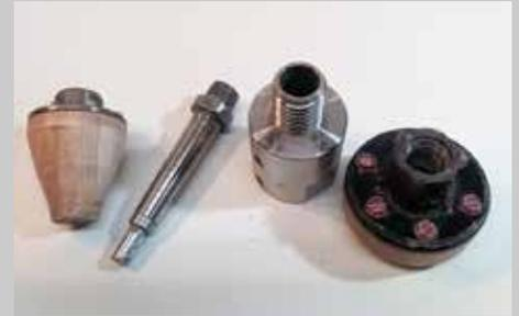
A Morse taper adapter (left center) and spindle adapter (right center) allow for the use of small faceplates on a larger lathe.
